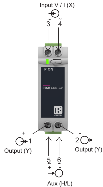
Fig. 3. RISH CON - CV/CA Connection Diagram.
